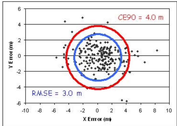
Figure 2. Horizontal accuracy of Ikonos image basemaps from 210 independent check points derived from rapid-static GPS survey.
