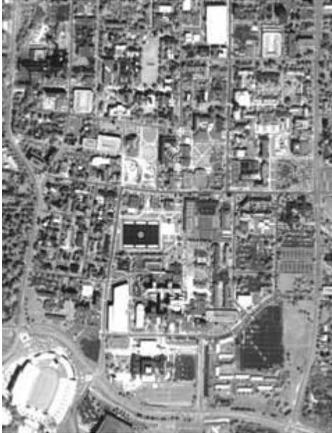
Figure 1. One meter resolution Ikonos image basemap of MU campus. The horizontal accuracy is about 4 m CE90.
