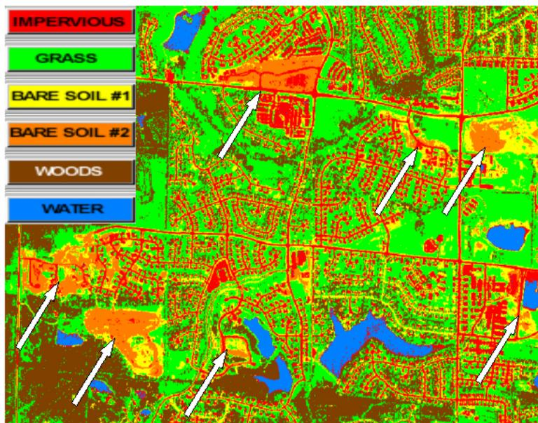
Figure 5. Result of supervised maximum likelihood classification with six classes. Areas with active construction sites shown by arrows.
