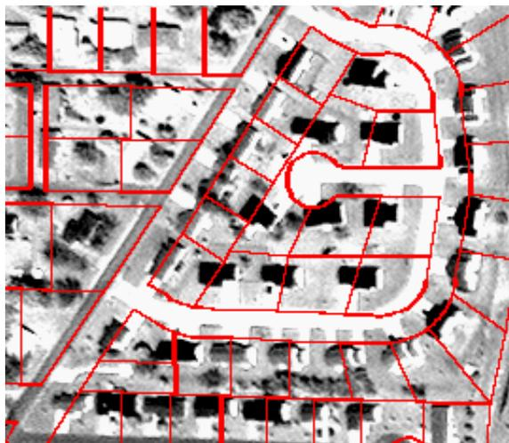
Figure 1: Typical Example of Vector Overlay on Imagery
