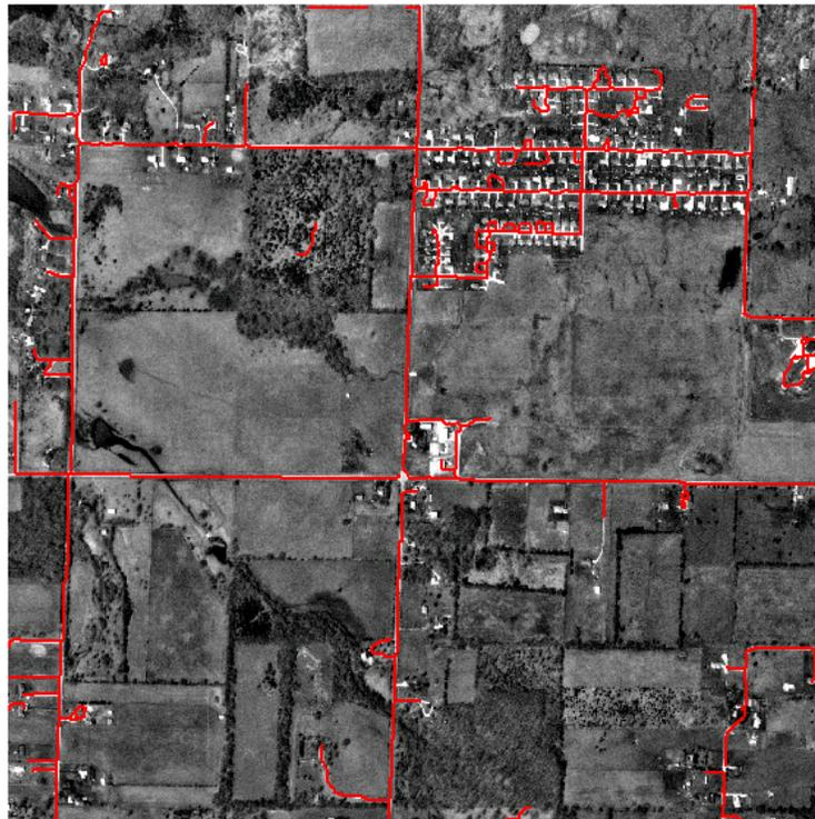
Figure 4. Extracted roads (red) from a DOQ image
