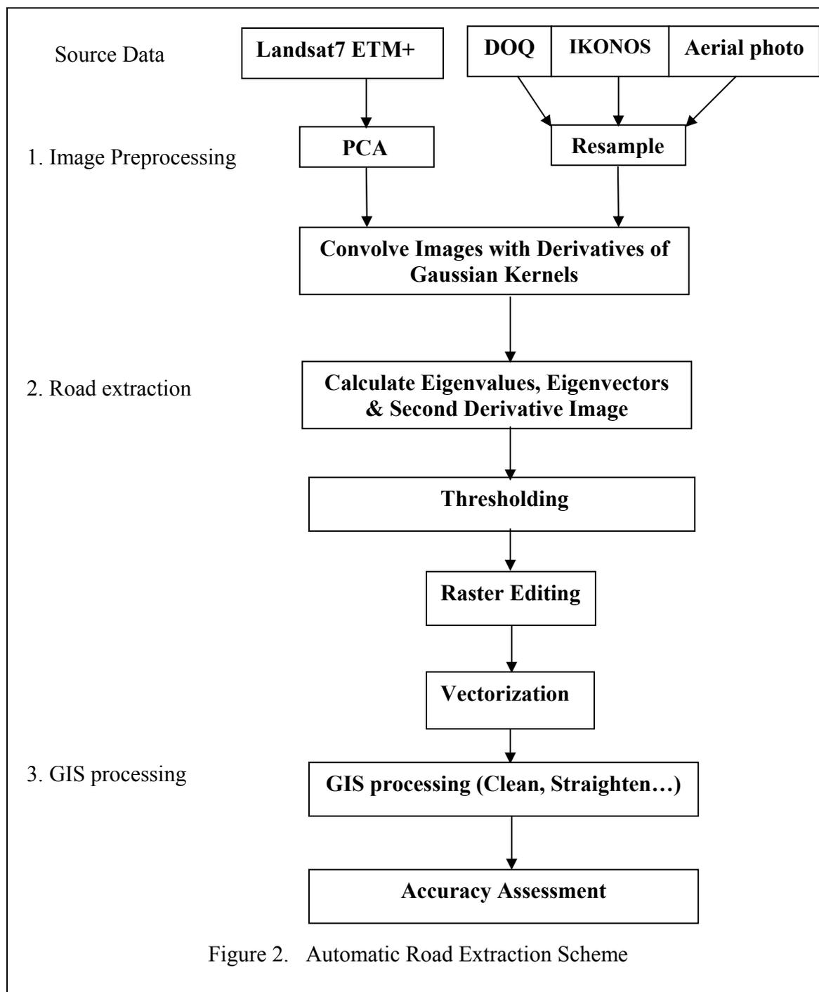
Figure 2. Automatic Road Extraction Scheme
